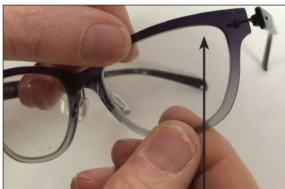
Bevel edged forward to be flush with the frame front
